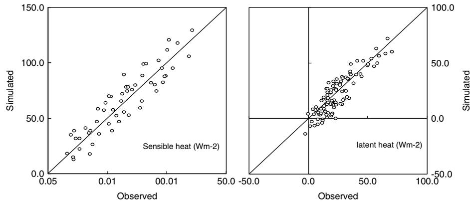
Figure 7. Simulated versus measured daily latent heat and sensible heat flux from 20 May to 29 August 2004
