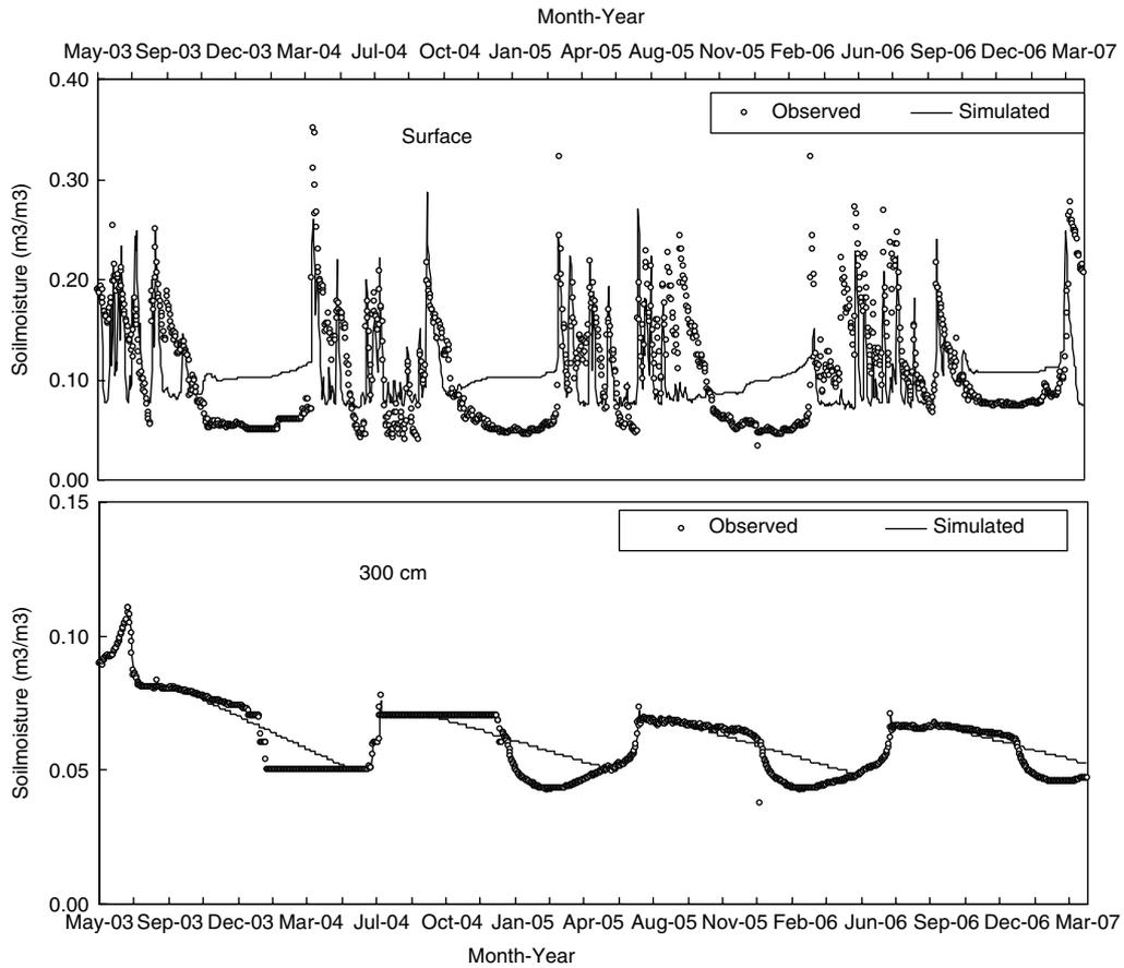
Figure 5. Simulated *versus* measured average daily soil moisture ( $\text{m}^3/\text{m}^3$ ) at depths of 0-0 and 3-0 m
