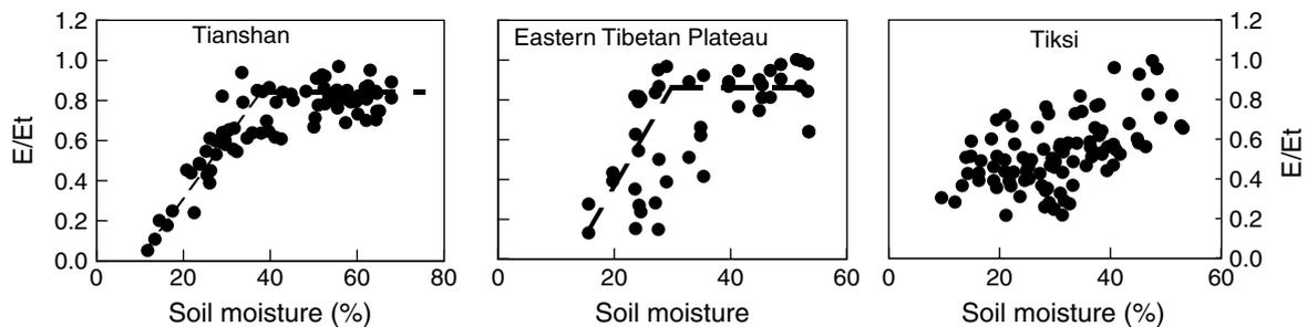
Figure 3. The variation of evaporation efficiency versus surface soil moisture at sites in the Tianshan Mountains, on the eastern Tibetan Plateau, and at Tiksi, eastern Siberia
