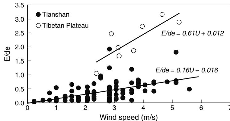
Figure 4. The ratio of daily sublimation to saturation deficiency  $E/De$  versus daily mean wind speed in the Tianshan region and on the eastern Tibetan Plateau
