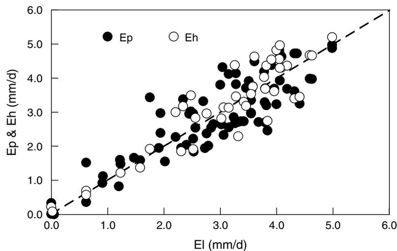
Figure 2. Comparison of daily evaporation observed by the profile method ( $E_p$ ) or heat budget method ( $E_h$ ) versus lysimeter results at the Tianshan site
