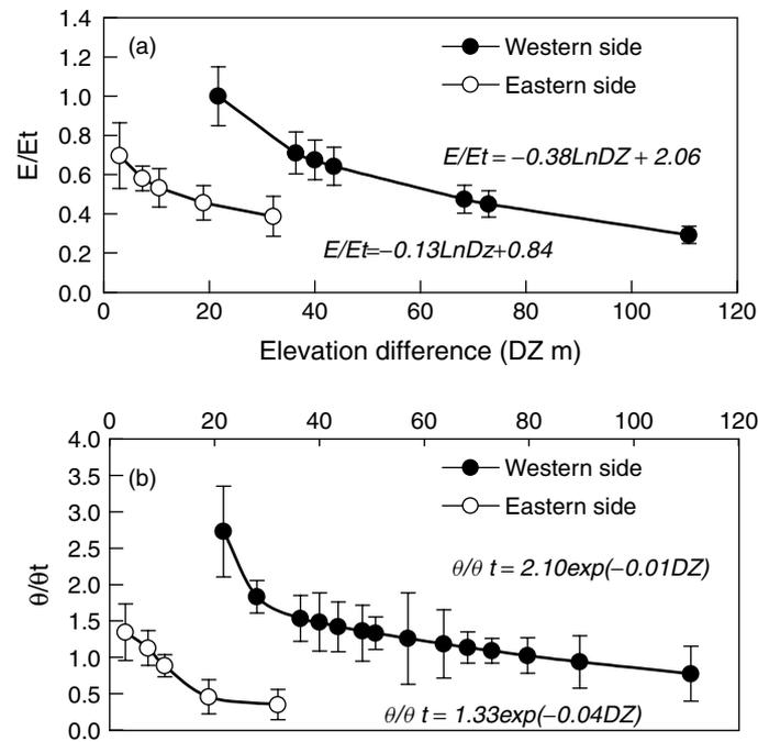
Figure 5. Variation of ratio of daily evaporation to potential evaporation  $E/E_t$  versus elevation difference (a) and ratio of soil moisture to saturate moisture  $\theta/\theta_t$  versus elevation difference at the Tiksi network
