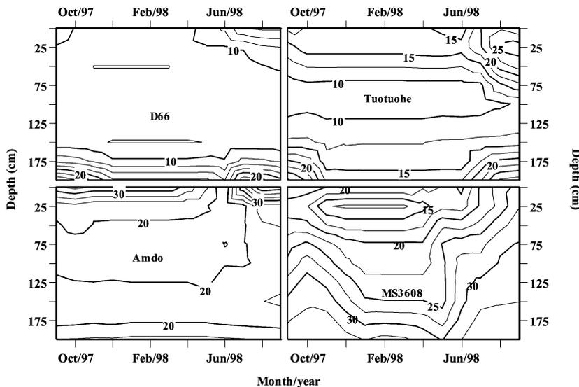
Fig. 3. Contours of the monthly mean soil volumetric water content (%) at all the study sites on the eastern Tibetan Plateau.
