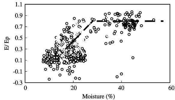
Fig. 5. The ratio of daily evaporation to daily potential evaporation ( $E/E_p$ ) versus surface moisture.
