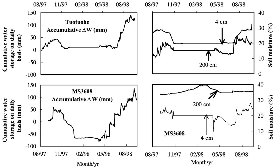
Fig. 6. Seasonal variation in the cumulative daily change in water storage and daily mean soil moisture measured at the surface and bottom of the study layer at Tuotuohe (continuous permafrost) and MS3608 (discontinuous permafrost) on the eastern Tibetan Plateau.
