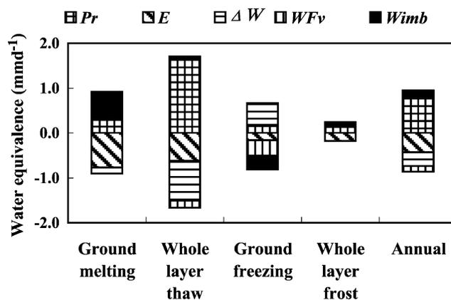
Fig. 9. The composition of the water budget in the ground surface layer (0–200 cm) at Tuotuohe on the eastern Tibetan Plateau.
