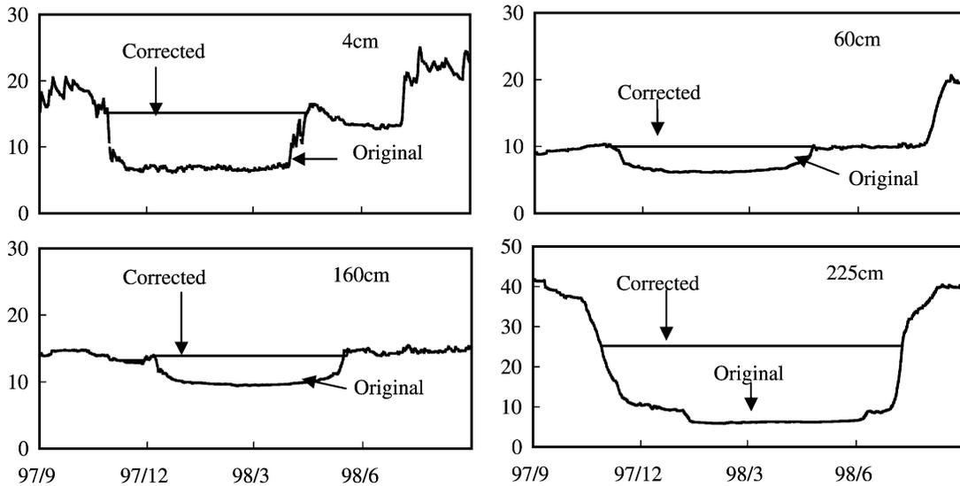
Fig. 1. Comparison of the original soil moisture data measured by TDR and the corrected value for the Tuotuohe site.
