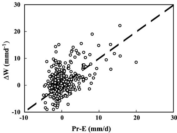
Fig. 7. The daily variation in water storage at 0–200 cm depths ( $\Delta W$ ) versus the difference between daily precipitation and evaporation ( $P_r - E$ ) in a region underlain by permafrost.
