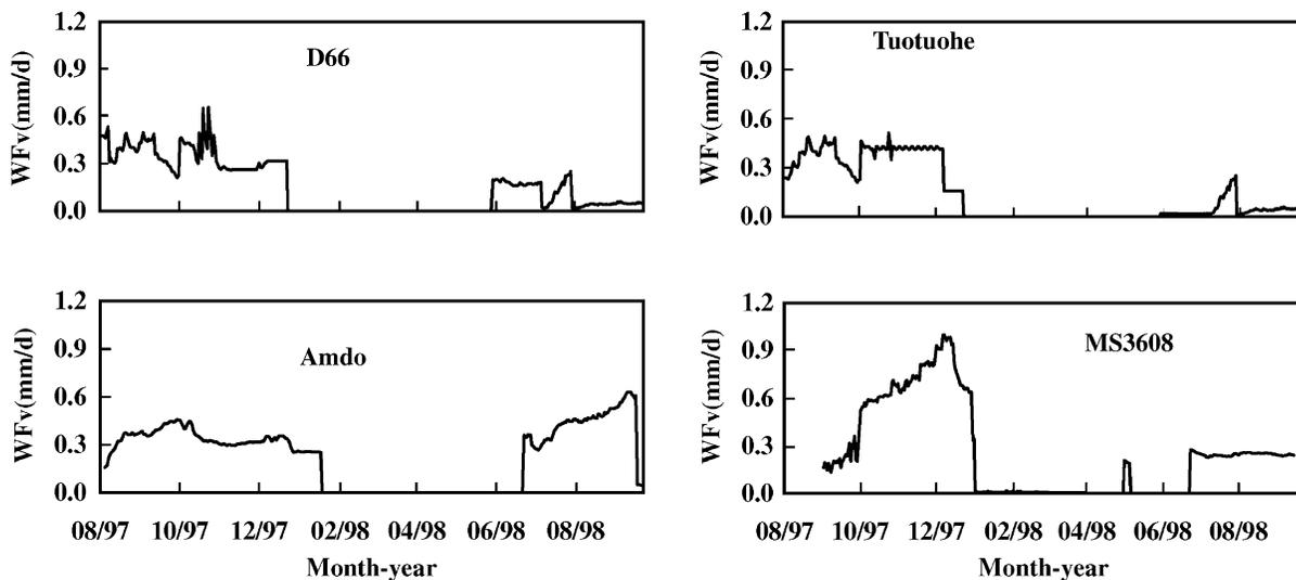
Fig. 8. Seasonal variation in the daily vertical water flux ( $WF_V$ ) at the bottom of the study layer (200 cm at D66, Tuotuohe, and Amdo, and 190 cm at MS3608).
